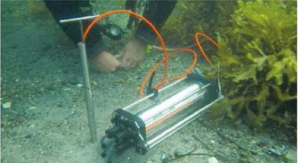
Fig. 23: The spear-like sediment profiler tested at Tudsø Hage.
