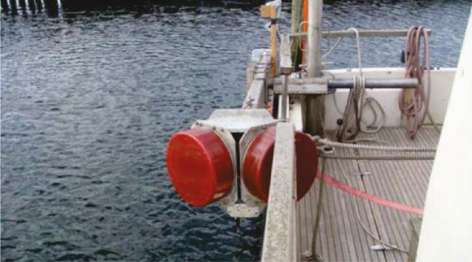
Fig. 2: Example of a MBES system
